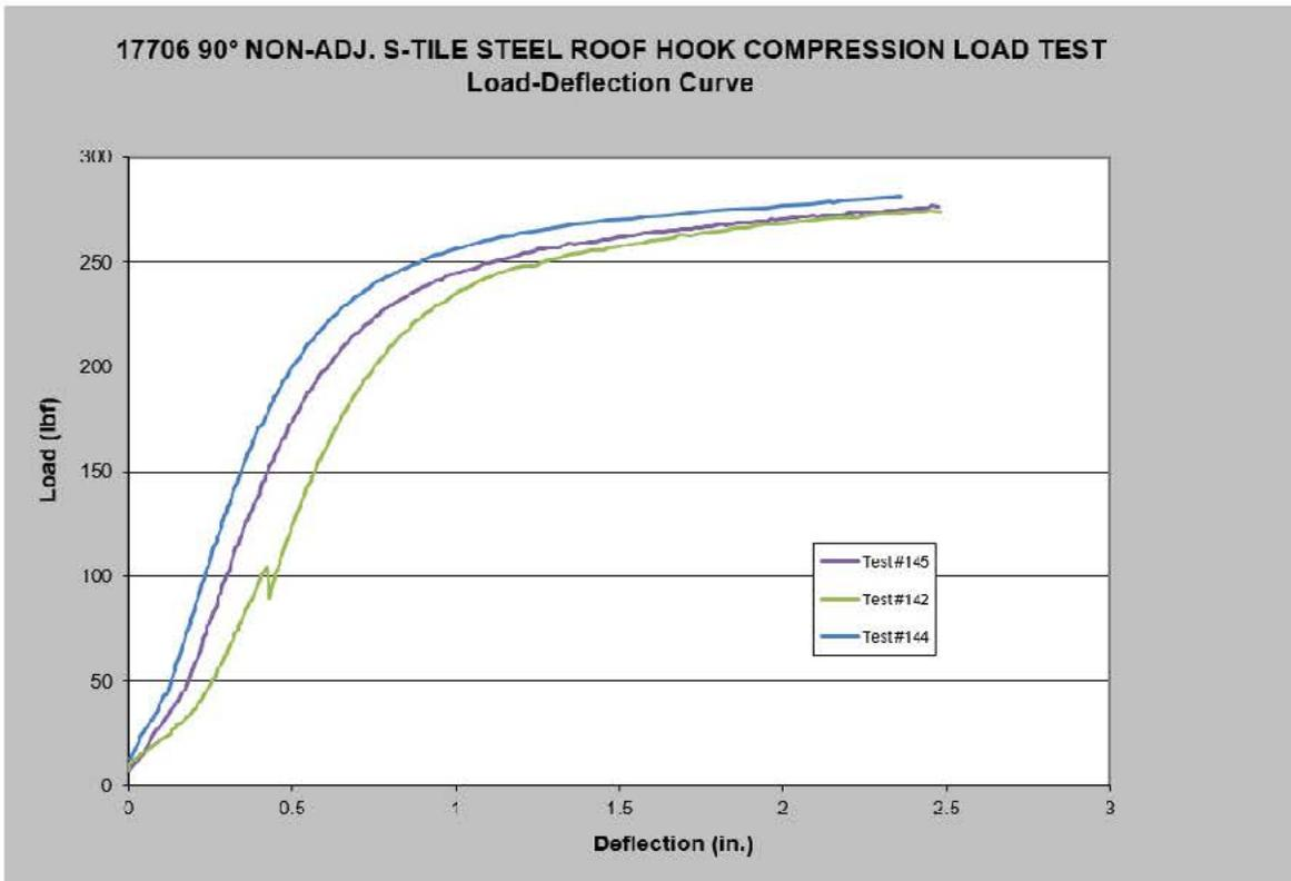
Note: Maximum deflection and peak load taken before sharp increase in load, when hook contacts plywood test board
